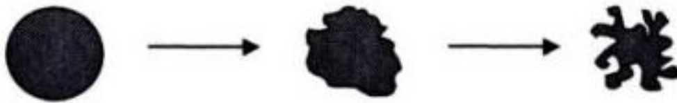
Fig 5. Surface Erosion of degradable polymer device, such as Checkmate.
